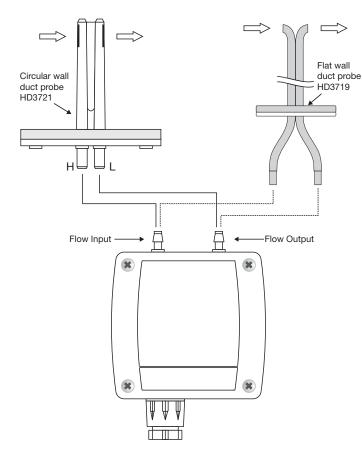
The outlet channel should be oriented so that the flow enters from the inlet connected to the junction on the left side of the housing and exits from the right side.
