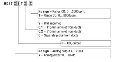
Order codes for CO<sub>2</sub> and temperature transmitters
