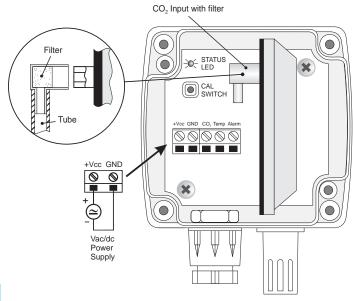
Open the instrument top cover to discover the CAL SWITCH calibration key on the board and the calibration gas inlet.
