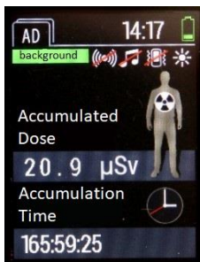
Figure 7 – Mode of DE measurement
