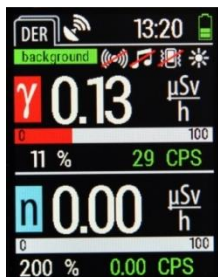
Figure 5 – Mode of DER measurement and indication
