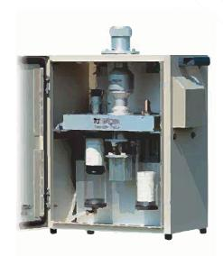
The modularity of the sampling head allows choosing the desired impactor type to operate in accordance with the EN 12341 and USEPA 40 CFR Part 50 methods.
